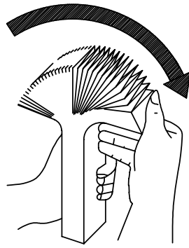
Fig. 5.5 Loosening the Chart Paper
