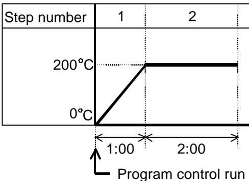
This program pattern shows that the temperature rises to 200°C for 1 hour and stays at 200°C for 2 hours. In this case, Step 1 step SV is 200°C and Step 1 step time is 1 hour.
