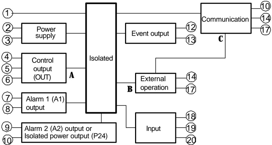
**When the control output is non-contact voltage output type or DC current output type, between A to B and A to C are not isolated.**
