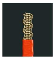
End Caps-Vulcanized fiber reinforced silicone rubber **Duo-Tape Element-**Double, knitted multi-strand Alloy, and two braided layers of **AMOX**<sup>M</sup> yarn
