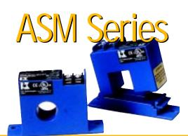
The 'ASM' Series Load Monitoring Switches from NK Technologies are designed for overload, underload or operating window applications. Upon sensing an average operating current, the ASM self-learns and establishes a limit-alarm trip point based on +/- 15% of the average expected current draw. The ASM offers a choice of solid state outputs and is available in solid or split-core enclosure styles.
