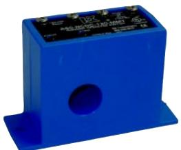
'ASO' Low-Current Sensors from NK Technologies are specialized current operated switches which combine an ultra-sensitive current transformer and signal conditioning electronics into a single package for sensing AC current from 3-350mA. Useful for signal or lamp status monitoring, detecting minute fault currents or fan proving, the ASO features solid-state outputs and jumper-selectable ranges, which make it a versatile choice for low-current status indicating applications.
